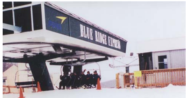
Upgrade at Wintergreen. The new $6M detachable lift gets you and five companions to the top in 3 minutes. The rest of the Division is jealous!
